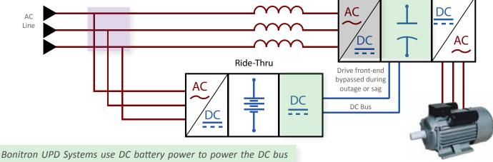
of the drive via DC bus connection terminals on the drive. This eliminates an unnecessary and energy wasting DC to AC conversion.
